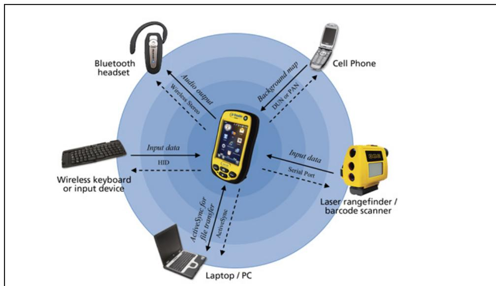
Figure 1.4 Juno series handheld Bluetooth client connections
