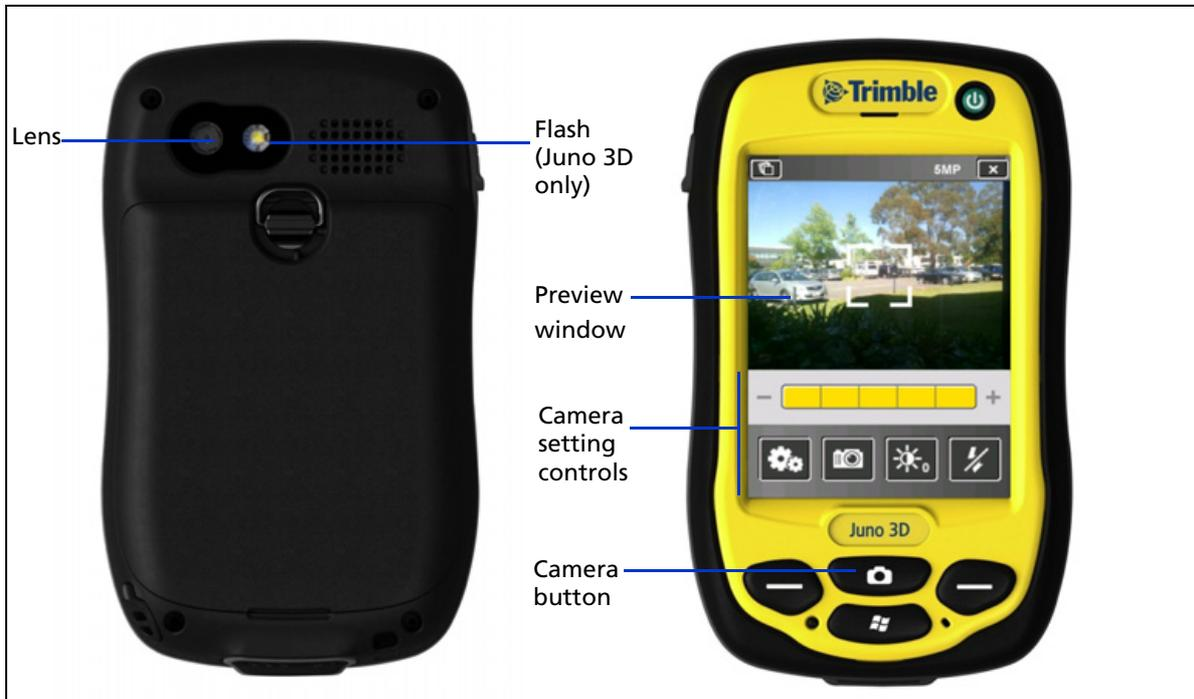
Figure 1.5 Juno series handheld – camera controls
